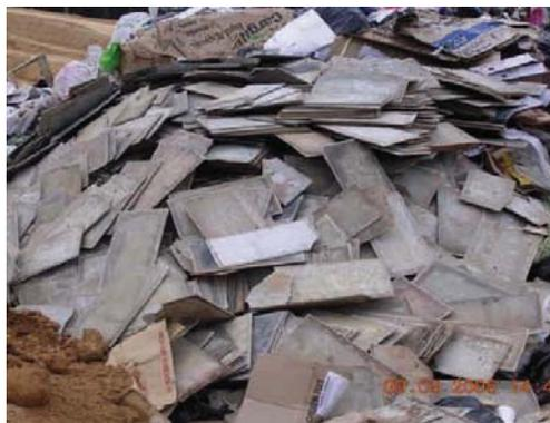
Figure 2: Bonded Asbestos Tiles
