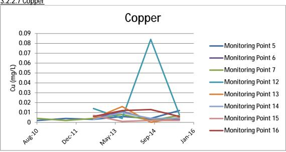
Results from this sampling period show that Copper is present in minor concentrations which are quite low. Monitoring point 12 has returned to the lower levels following the spike in September 2014.
