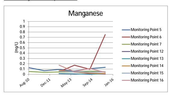
The 2011 Australian Drinking Water Guidelines 6 states that a maximum of 0.5 mg/L of manganese is safe for consumption. Manganese can be a strong indicator of landfill leachate in groundwater leached from hazardous waste sites and often derived from battery disposal. Monitoring point 6 is 0.75mg/l, and has started to rise this will need to be watched before the rehabilitation program begins in 2016/17
