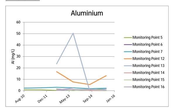
Aluminium levels in the sampled groundwater monitoring wells have traditionally been maintained at a consistent low level. However, relative higher levels of aluminium detected in Monitoring Points 12 and 13 in 2013 which both represent the groundwater flow prior to intercepting the former landfill site. Anthropogenic sources of aluminium in groundwater are generally related to low pH runoff and colliery based leachate.
