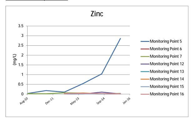
The 2011 Australian Drinking Water Guidelines 6 states that for aesthetic reasons a maximum of 3 mg/L of zinc is desirable for consumption. Landfill sites can be an anthropogenic source of zinc in groundwater, however the extremely low levels of zinc detected indicate that landfill leachate is not intercepting the groundwater system around the site. Monitoring Point 5 is showing a steady increase, however this Sample Point is upstream of the landfill in respect to the flow of groundwater.
