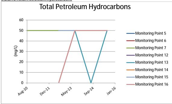
Total Petroleum hydrocarbons have not risen above the 50mg/L since testing commenced, this year is in line with this upper limit.
