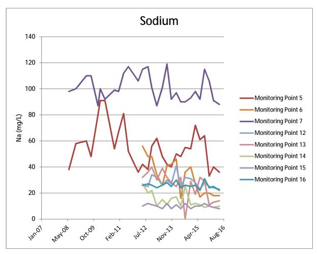
The trend for sodium has been below 120mg/L over the history of available results. High sodium levels are another indicator of leachate infiltrating the groundwater. The 2011 Australian Drinking Water Guidelines 6 set a maximum level of sodium in drinking water at 180mg/L for aesthetic reasons. The sodium results experienced in the groundwater at Helensburgh indicate that the groundwater is not contaminated by leachate.
