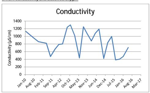
Conductivity is a measure of the waters ability to pass electrical current, usually though positively or negatively charged inorganic dissolved solids (e.g. sodium, magnesium, calcium, iron). The conductivity results for the Pony Club pond have been slowly rising in this reporting period in line with previous trends, these will continue to be closely monitored.
