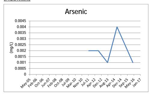
There are low levels of Arsenic in the Leachate Pond. Arsenic found in the surrounding boreholes is in line slightly higher than the leachate pond but not consistent enough to say it is from the leachate.
