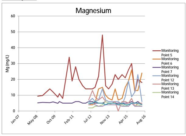
Groundwater monitoring well results are in line with historical levels and have maintained consistent levels with the exception of point 5, which is located up gradient of the site. However, point 5 is still considered to be at relative low levels. The magnesium levels sampled would be considered 'soft' in the 0-60mg/L area. 'Hard' water would be considered in the region of 120-180mg/L.
