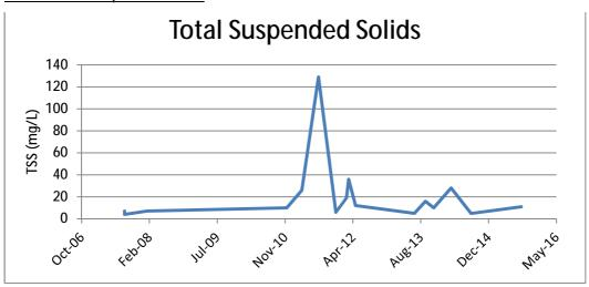
Apart from an individual spike in July 2011, the onsite stormwater treatment meets EPL requirements, the result from the 26 August 2015 was measured at 11mg/l.
