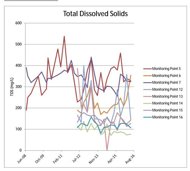
The 2011 Australian Drinking Water Guidelines 6 states that total dissolved solids levels of less than 600mg/L indicate good quality drinking water. The dissolved solids levels in the groundwater monitoring wells are in line with historical trends. Monitoring point 6 is starting to trend up and this will need to be monitored in the following years data. High levels of dissolved solids can be sourced from salts derived from leachate infiltration.
