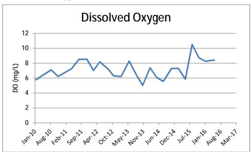
Dissolved oxygen levels can be depleted by biological activity associated with the nitrification process (common in leachate). The dissolved oxygen levels have started to taper down toward historic levels, the following years monitoring will need to be reviewed closely to ensure that the data continues to trend in the historic ranges.
