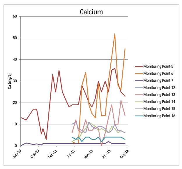
The groundwater monitoring wells show individually stable trends for calcium levels. The calcium levels sampled would be considered 'soft' in the 0-60mg/L area. 'Hard' water would be considered in the region of 120-180mg/L.
