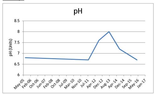
pH levels in the leachate pond have remained stable over a relatively long sample period. The pH averages around 7.5 which would foster the aerobic nitrification process in the leachate.
