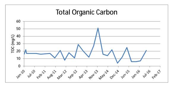
Microbial degradation of organic matter can increase the total organic carbon content in water and may provide evidence of contamination by natural compounds derived from the landfilling of organic matter. The amount of total organic carbon during this reporting period has remained within historical ranges.
