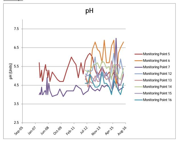
The pH levels indicated in the groundwater monitoring wells range from 4-7 units. The relatively low pH found naturally in the groundwater on site give an increased propensity for heavy metals to breakdown and travel through the system. The rehabilitation program is scheduled for 2016/17.
