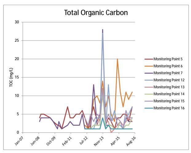
Microbial degradation of organic matter can increase the total organic carbon content in water and may provide evidence of groundwater contamination by organic compounds derived from the landfilling of organic matter. Data from the reporting period shows a similar slight rising trend, this will need to be observed to ensure that there is no pattern emerging. It should also be noted that organic materials have not been landfilled at the Helensburgh site since 1991.
