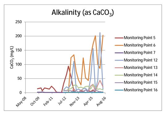
Increased alkalinity levels can be caused by many chemical processes including the denitrification process common in landfill leachate. Denitrification is the anaerobic biological reduction of nitrate ( $NO_3$ ) to nitrogen ( $N_2$ ) in its gaseous form. Under anoxic conditions microorganisms consume the oxygen in the nitrate and liberate the nitrogen. This process produces calcium carbonate as a byproduct.
