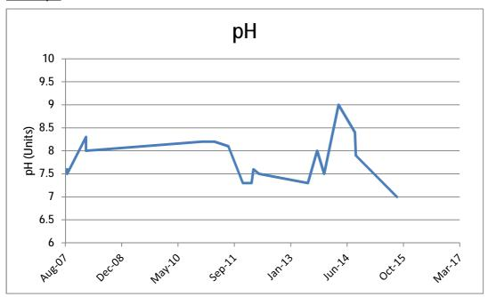
The pH derived from onsite stormwater has traditionally performed well within EPL requirements. The pH has sample taken during the reporting period returned a reading of 7 which is within the specified range.
