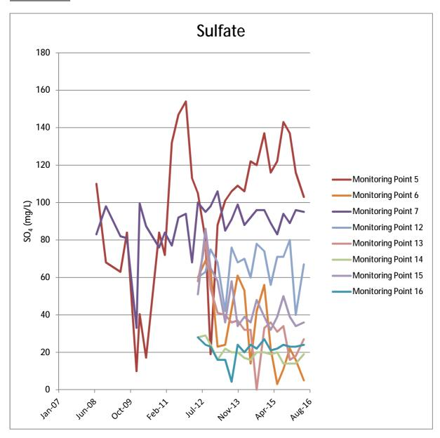
The 2011 Australian Drinking Water Guidelines 6 sets maximum sulfate levels in drinking water as 500mg/L. The sulfate levels in the groundwater monitoring wells are in line with the historical levels and are below the drinkable water maximum standard. Inorganic ions such as sulfate provide a good indication of groundwater contamination by landfill leachate. A sudden increase in these ions can act as early warning system.
