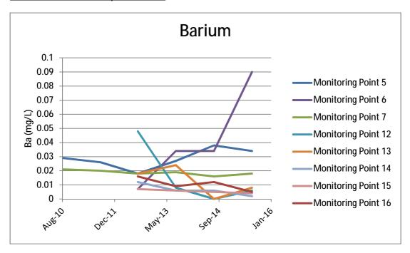
The 2011 Australian Drinking Water Guidelines 6 states that a maximum of 2 mg/L of barium is safe for consumption. Anthropogenic sources of barium in groundwater include bleaches, dyes and drillers mud. Barium levels are therefore extremely low and relatively stable in the sites groundwater, monitoring point 6 will need to be monitored as it is rising sharply.
