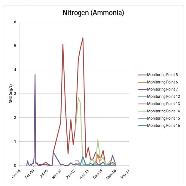
The groundwater monitoring wells for this reporting period show that the results are tracking the same as previous years. The relatively low results for ammonia in down gradient Monitoring Points indicate that the groundwater departing the site is not affected by Ammonia, which is perhaps the clearest signature of leachate.
