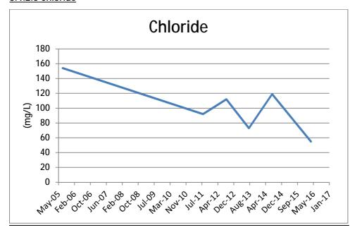
Chloride sampling has been showing a downward trend, which has been continuing into this sampling period.
