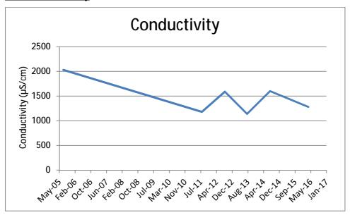
Electrical conductivity levels are higher than the surrounding stormwater pond, suggesting that leachate is being effectively contained and treated.
