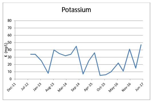
Potassium is present in bodies of water outside coastal areas generally through weathering of clays and agricultural purposes (leaching of fertiliser). Potassium levels have fluctuated between approx. 5-47mg/l over 5 years of sampling, this year's data is in line with previous data.
