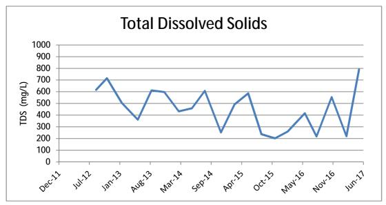
The 2011 Australian Drinking Water Guidelines 6 states that total dissolved solids levels of less than 600mg/L indicate good quality drinking water. High levels of dissolved solids can be sourced from salts derived from leachate infiltration. The samples taken indicate that the pond continues to demonstrate mild fluctuations between 200-800 mg/L.
