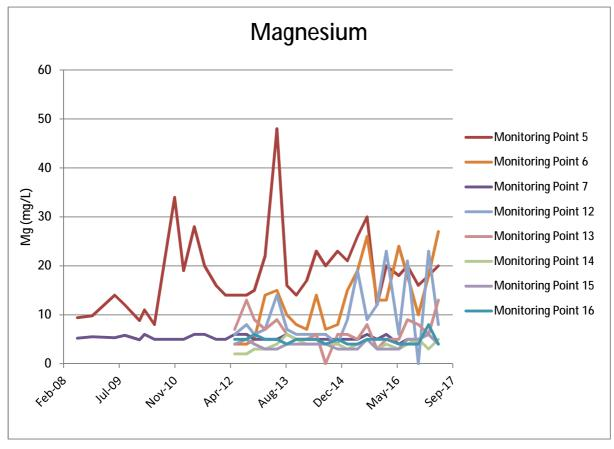
Groundwater monitoring well results are in line with historical levels and have maintained consistent levels with the exception of point 5 (located up gradient of the site) and Point 6 (located east of the pony club site). However, point 5 & 6 are still considered to be at relative low levels. The magnesium levels sampled would be considered 'soft' in the 0-60mg/L area. 'Hard' water would be considered in the region of 120-180mg/L.
