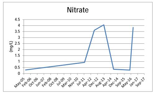
Nitrate sampling peaked in August 2013, Nitrate levels have returned a higher reading in borehole 15. Nitrate levels have been between the ranges of 0.9 – 4 over the past years and this is in line with that range.
