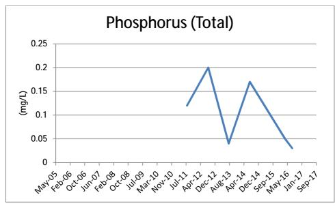
Phosphorus has been erratic in the past sampling, however all at low levels. This sampling period has returned levels consistent with a downward trend.
