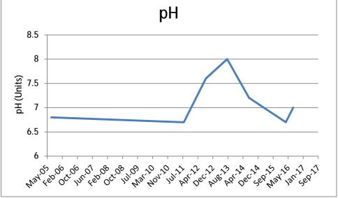
pH levels in the leachate pond have remained stable over a relatively long sample period. The pH averages around 7.5 which would foster the aerobic nitrification process in the leachate.
