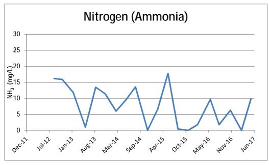
The trend for Nitrogen as Ammonia has been ultimately stable over time fluctuating at a maximum between 2 and 18 mg/L. This sampling period is well within that expected range. Therefore, there is no indication that leachate is entering the pond.
