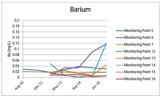
The 2011 Australian Drinking Water Guidelines 6 states that a maximum of 2 mg/L of barium is safe for consumption. Anthropogenic sources of barium in groundwater include bleaches, dyes and drillers mud. Barium levels are therefore extremely low and relatively stable in the sites groundwater.
