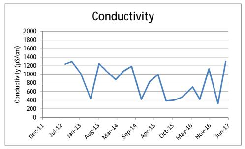
Conductivity is a measure of the waters ability to pass electrical current, usually though positively or negatively charged inorganic dissolved solids (e.g. sodium, magnesium, calcium, iron). The conductivity results for the pond have fluctuated consistently within the range of approximately  $1,000\mu$ S/cm for the last 5 years.
