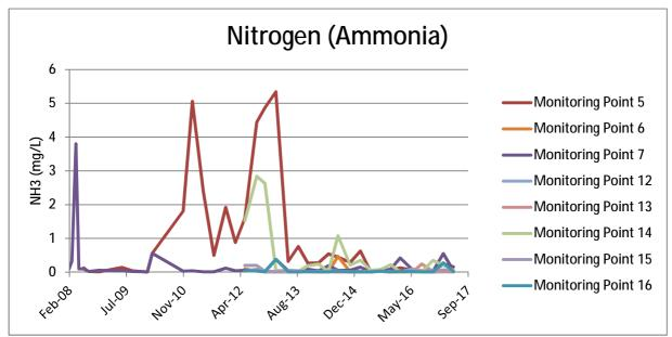
The groundwater monitoring wells for this reporting period show that the results are tracking in line with expectations derived from previous years data. The relatively low results for ammonia in down gradient Monitoring Points indicate that the groundwater departing the site is not affected by Ammonia, which is perhaps the clearest signature of leachate.
