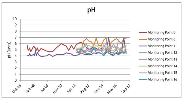
The pH levels indicated in the groundwater monitoring wells range from 4-7 units. The relatively low pH found naturally in the groundwater on site give an increased propensity for heavy metals to breakdown and travel through the groundwater system.
