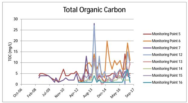
Microbial degradation of organic matter can increase the total organic carbon content in water and may provide evidence of groundwater contamination by organic compounds derived from the landfilling of organic matter. It should also be noted that organic materials have not been landfilled at the Helensburgh site since 1991.
