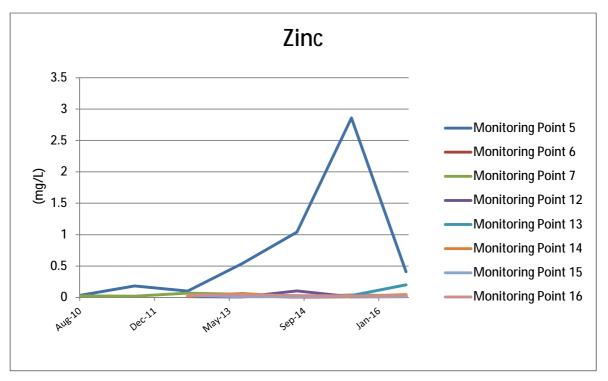
The 2011 Australian Drinking Water Guidelines 6 states that for aesthetic reasons a maximum of 3 mg/L of zinc is desirable for consumption. Landfill sites can be an anthropogenic source of zinc in groundwater, however the extremely low levels of zinc detected indicate that landfill leachate is not intercepting the groundwater system around the site. Monitoring Point 5 is showing a rapid decrease. This sample Point is upstream of the landfill in respect to the flow of groundwater.
