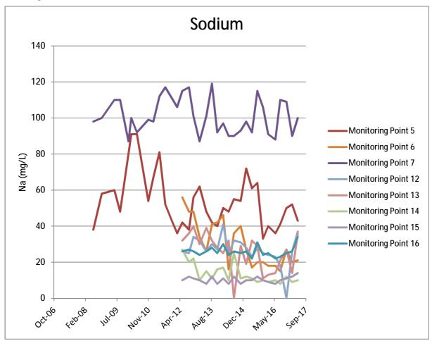
The trend for sodium has been below 120mg/L over the history of available results. High sodium levels are another indicator of leachate infiltrating the groundwater. The *2011 Australian Drinking Water Guidelines 6* set a maximum level of sodium in drinking water at 180mg/L for aesthetic reasons. The sodium results experienced in the groundwater at Helensburgh indicate that the groundwater is not contaminated by leachate.
