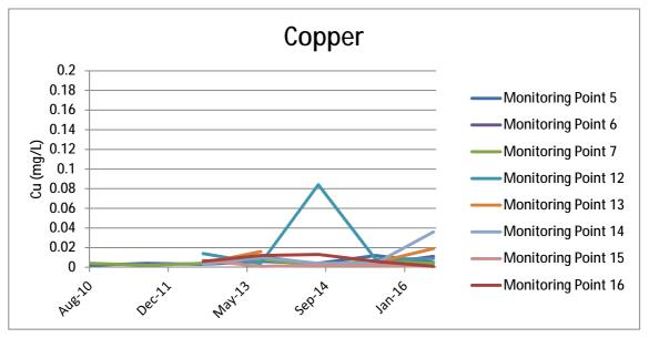
Results from this sampling period show that Copper contamination levels are extremely low. Monitoring point 12 has returned to the lower levels following the elevated result in September 2014.
