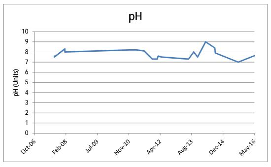
The pH derived from onsite stormwater has been consistent within "normal" ranges for pH. The pH was elevated slightly in March 2014 but has since returned to expected levels.
