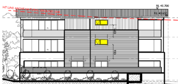
Figure 10: Eastern elevation of RFB with U13 and U20 windows highlighted
