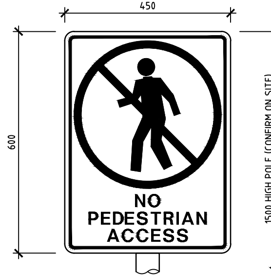
S9 CAR PARK SIGNAGE A801 NON-ILLUMINATED ALUMINIUM REFLECTIVE SIGN ON GALVANISED STEEL POLE TYPICAL.
