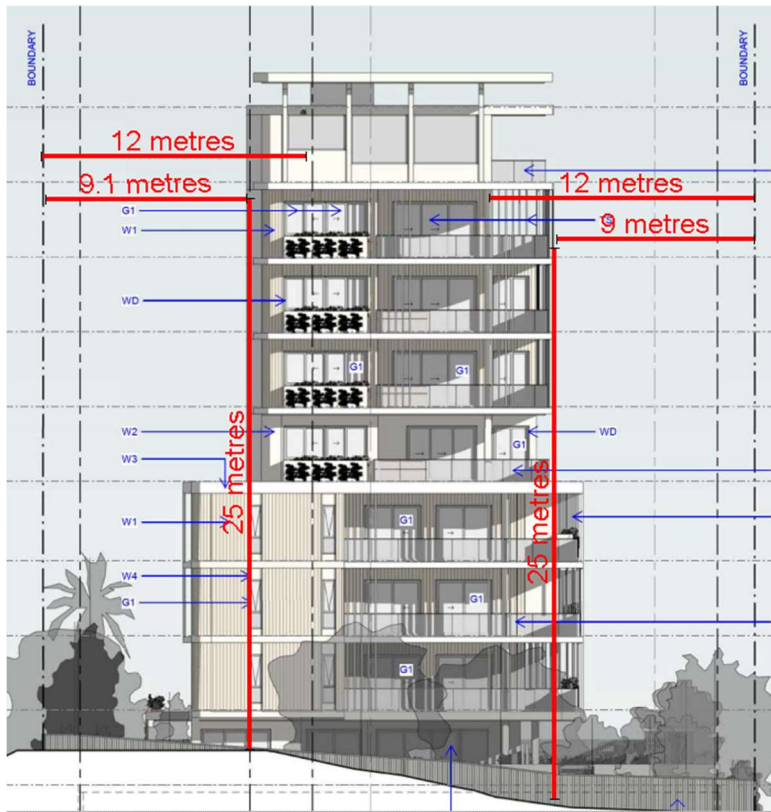
Figure 2: East elevation identifying non-compliant setback
