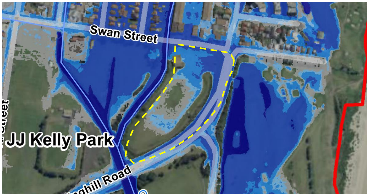
Figure 4-2 Extract from Wollongong City Flood Study (2019) Scenario ID2 "Design" blockage factor peak flood depth – 5% AEP event.
