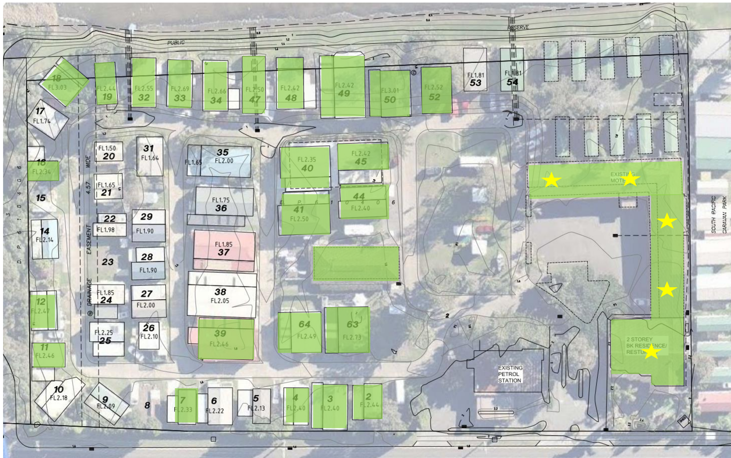
Extent of 1% AEP Refuge On-Site. Green Shading denotes existing FFL above the 2015 1% AEP flood level. Yellow star denotes PMF free FFL in the 2015 scenario.
