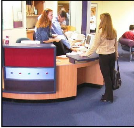
Figure 26: (Top left) Reception counters which allow for a frontal approach with an adequate toe plate and knee space for a person using a wheelchair.
