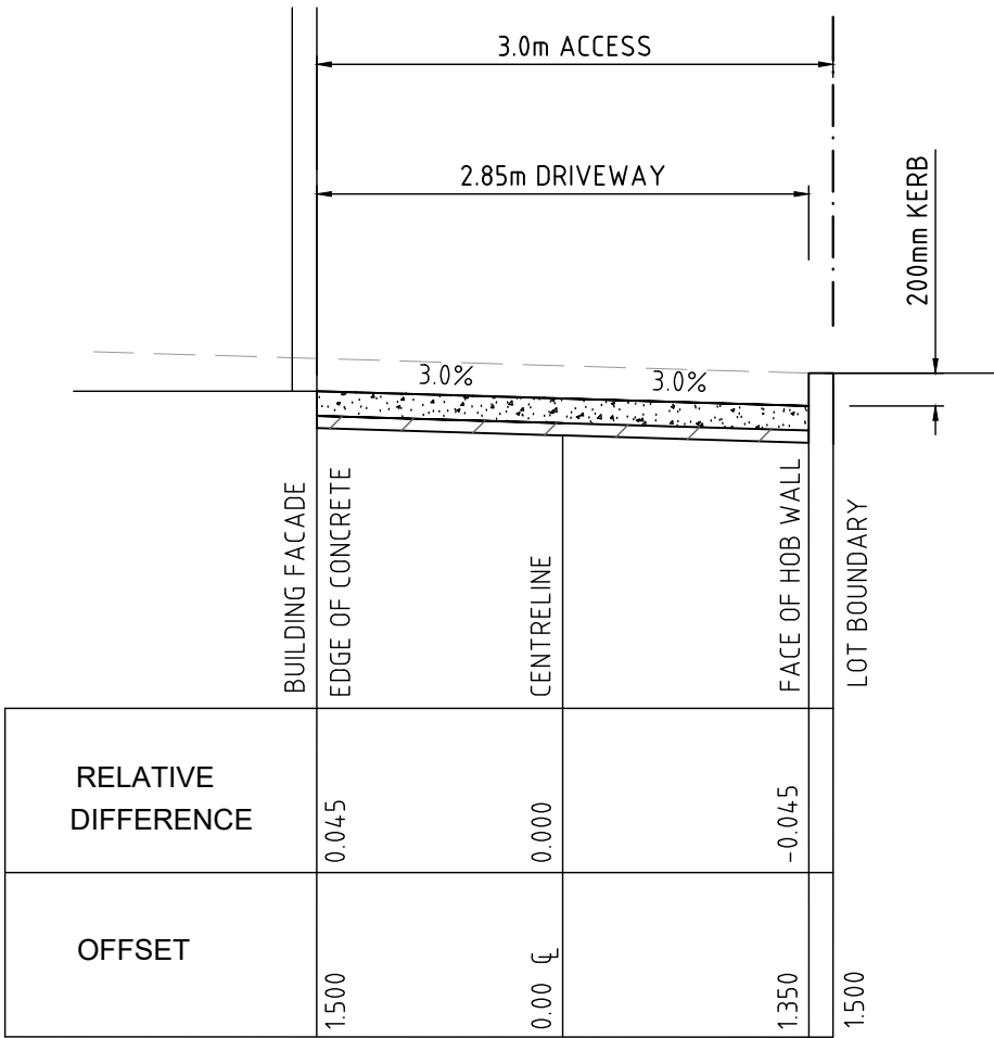
TYPICAL DRIVEWAY CROSS-SECTION SCALE 1:50
