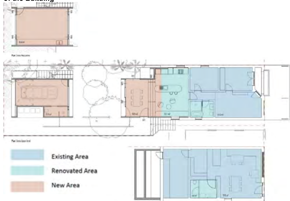
Figure 3.1 Floor plan showing existing, renovated and proposed portions of the Building
