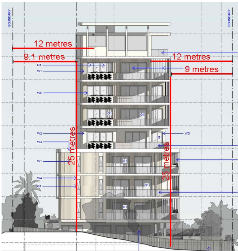
Figure 2: East elevation identifying non-compliant setback
