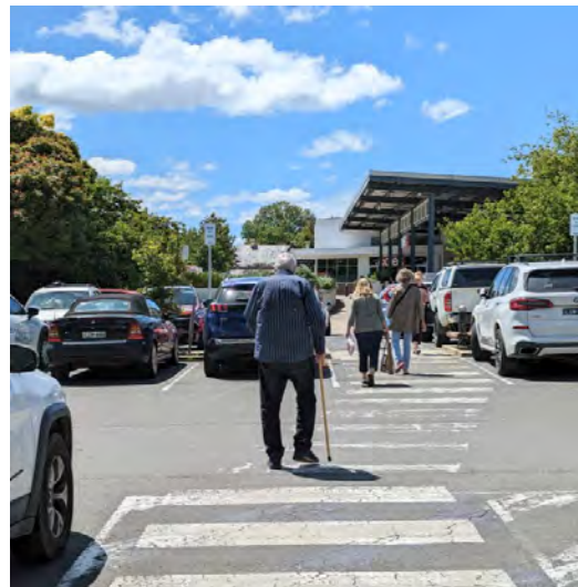
Figure 72: Clear and legible pedestrian links should be provided in car parking areas to ensure pedestrian safety and to enforce pedestrian priority.
