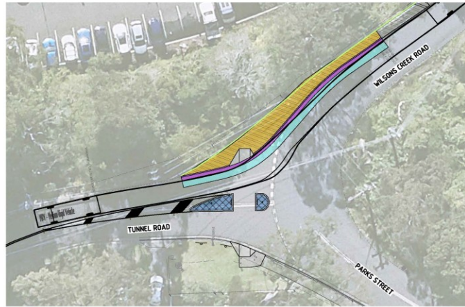
MEDIUM RIGID VEHICLE - 8.8m LENGTH - TURNING CHECK 1 (5km/h) SCALE 1:200
